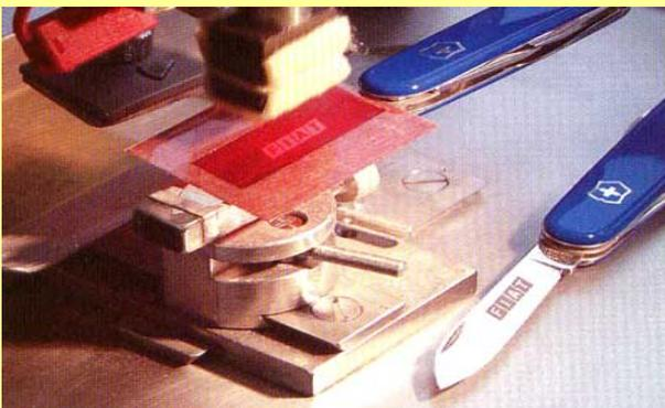
Inscriptions produced by electrolytic means (electrolyte and electric current).
