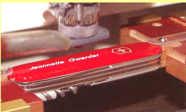
A tool mills the inscription into the material. If the material is plastic, the engraving is picked out with a contrasting color (white).
