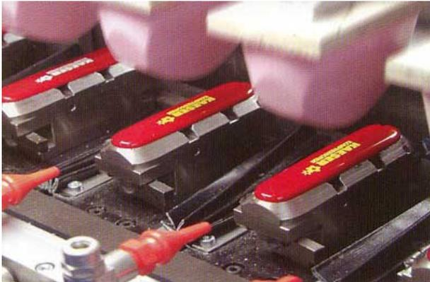
A silicone rubber stamp is used to transfer ink from the engraved steel printing block to the item which is to be printed.
