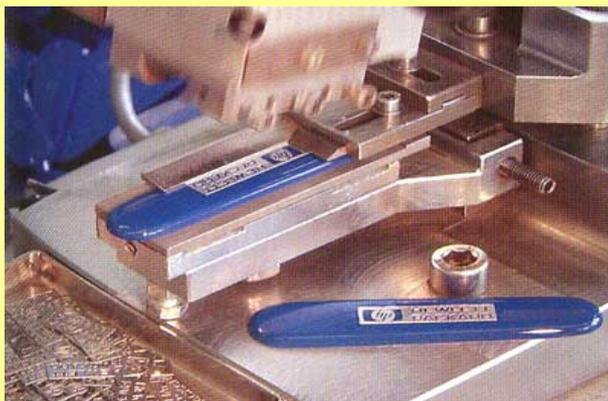
A chromium steel metal inlay is produced by means of photochemical techniques, and is then securely bonded into the plastic handle by heat and pressure (due to technical reasons, it is not possible for Nylon and translucent handles).
