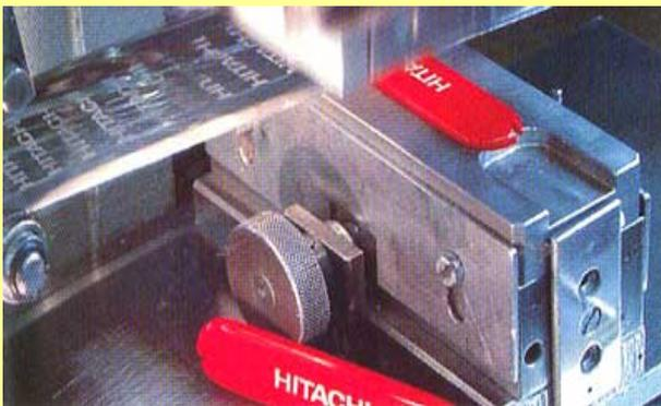
The design is impressed to a specific depth by means of a brass die-stamp, blocking foil, temperature and pressure. In contrast to the Tampoprint method, this is a dry printing process.
